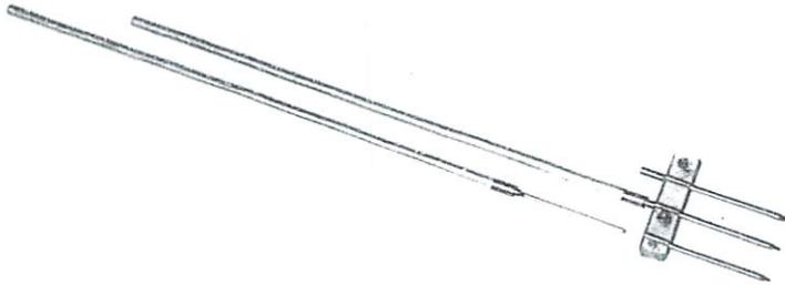
Fig. 43.—Demonstrating the activation of needles through a perspex stabilizer, using the handle.
