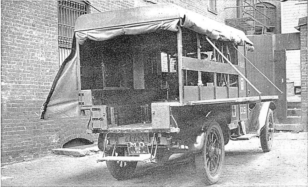
FIG. 9. AMERICAN CAMION WITH TABLE TOP ARRANGED FOR SLEEPING.
