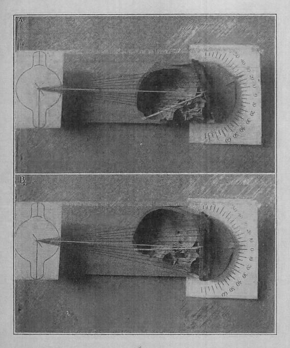
Two photographs of a model constructed for showing the effects of changing the position of the tube with reference to the skull. The direction of the rays in mesial plane is shown by stretched elastic cords passing from a point representing the target of tube to a bar placed in front of face and representing a line in the middle of plate. The principal ray is represented by a cord of lighter color than the others and the basal plane is shown by a strip of tape fastened to the skull at its base.
